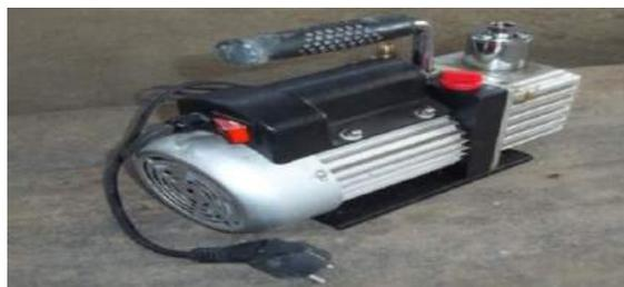
Gambar Pompa Vakum (Simbolon, F.,2014)
